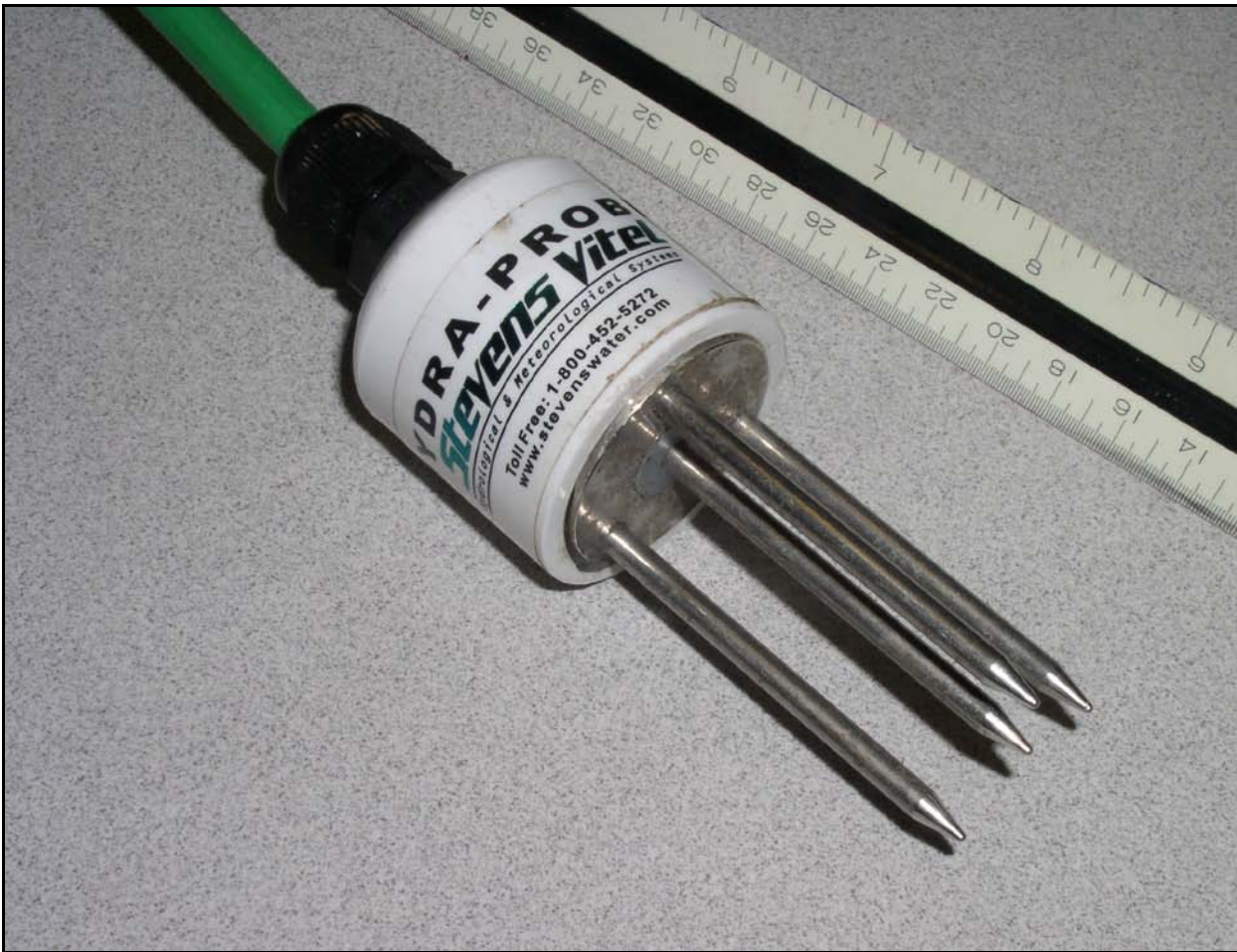
Example of hydraprobe used for collecting soil moisture and temperature data, along with other information. Five hydraprobes are installed in soil profiles at each site at 2, 4, 8, 20 and 40 inches below the surface.
