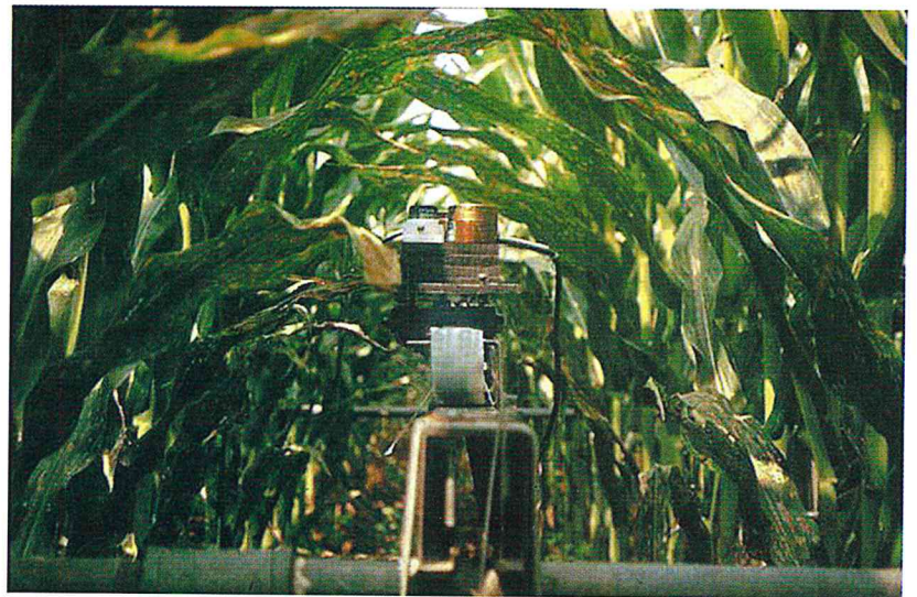
Below-canopy UV radiation sensors in a cornfield located at Purdue University's Agronomy Research Center.
