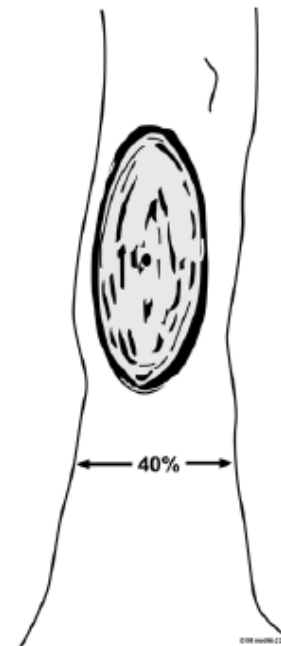
Figure 44. A canker which exceeds threshold. Since 40% of circumference is visible from any side, and since over half the visible side is taken up by the canker, it obviously exceeds the 20% minimum circumference threshold.
