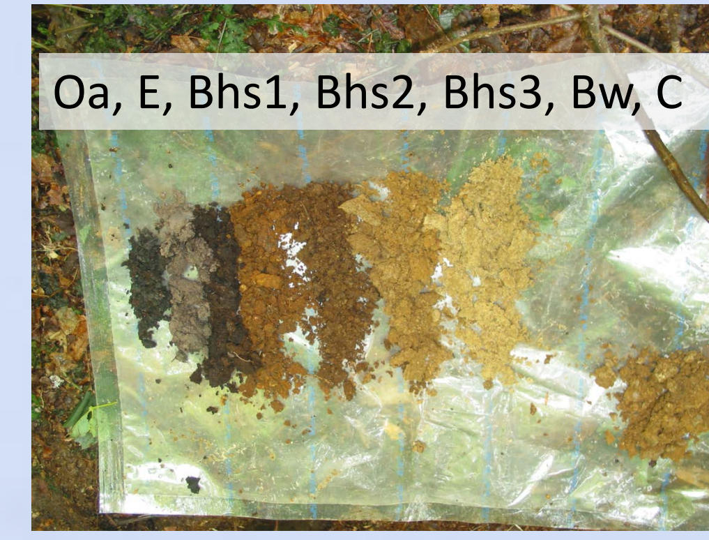
Podzol soil horizon sequence from the Lye Road site. THg was measured in the Oa horizon.
