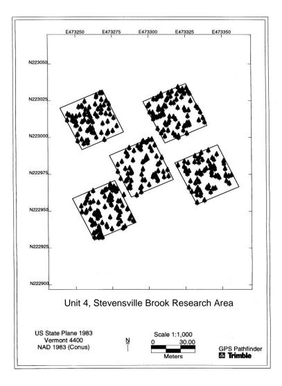
Figure 4. Surveyed tree positions in the five 0.1 ha. sampling plots located within one of the structural complexity enhancement units on the Stevensville Brook Research Area, Mount Mansfield State Forest, Vermont. Positions shown are for all trees > 5 cm diameter at 1.37 m ht. Tree positions have horizontal precisions ranging between 0.1 and 0.5 m with an average precision of 0.3 m.
