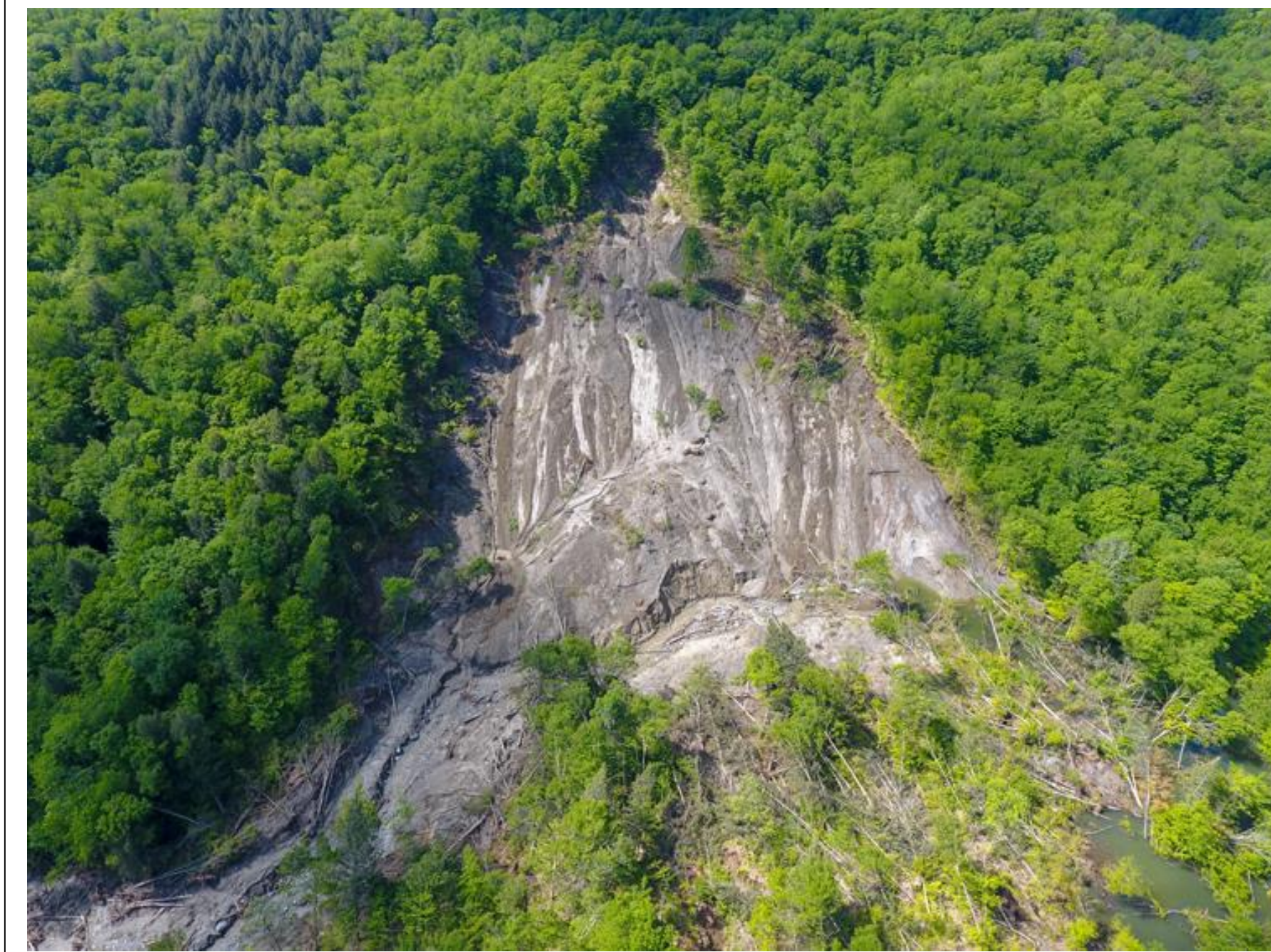
Fig 1. June 12, 2019: Drone flight by VTRANS showed 12 acres active plus 2.2 acres detached along the margins. ~100,000 cubic meters of material is in the toe deposit.
