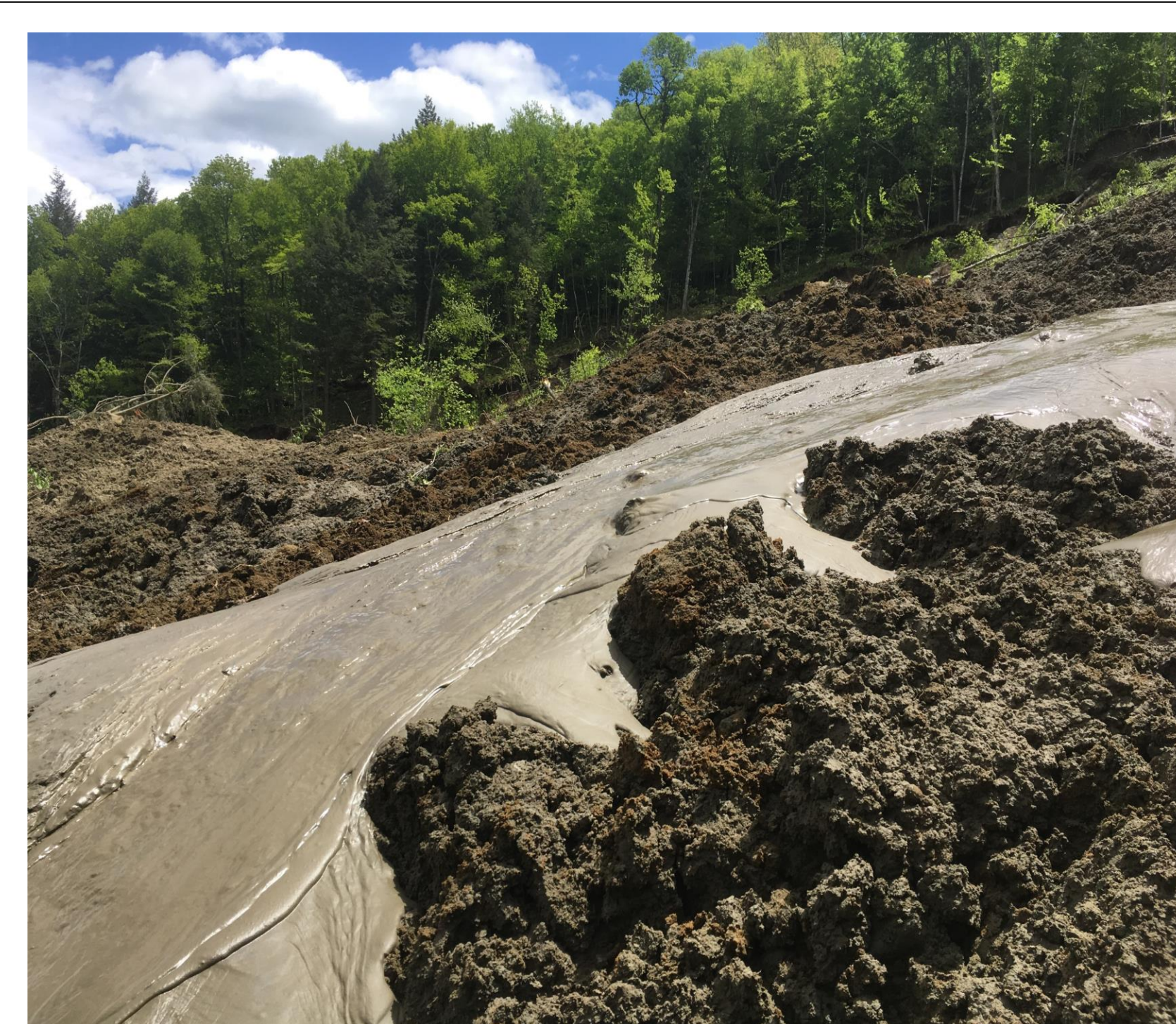
Fig. 6. June 4, 2019: Mudflows, saturated sand, boulders and trees indicated the site was still active. Water feeding the mudflows was from seeps partway down the slope, likely at a sand-silt interface or due to elevated water table.
