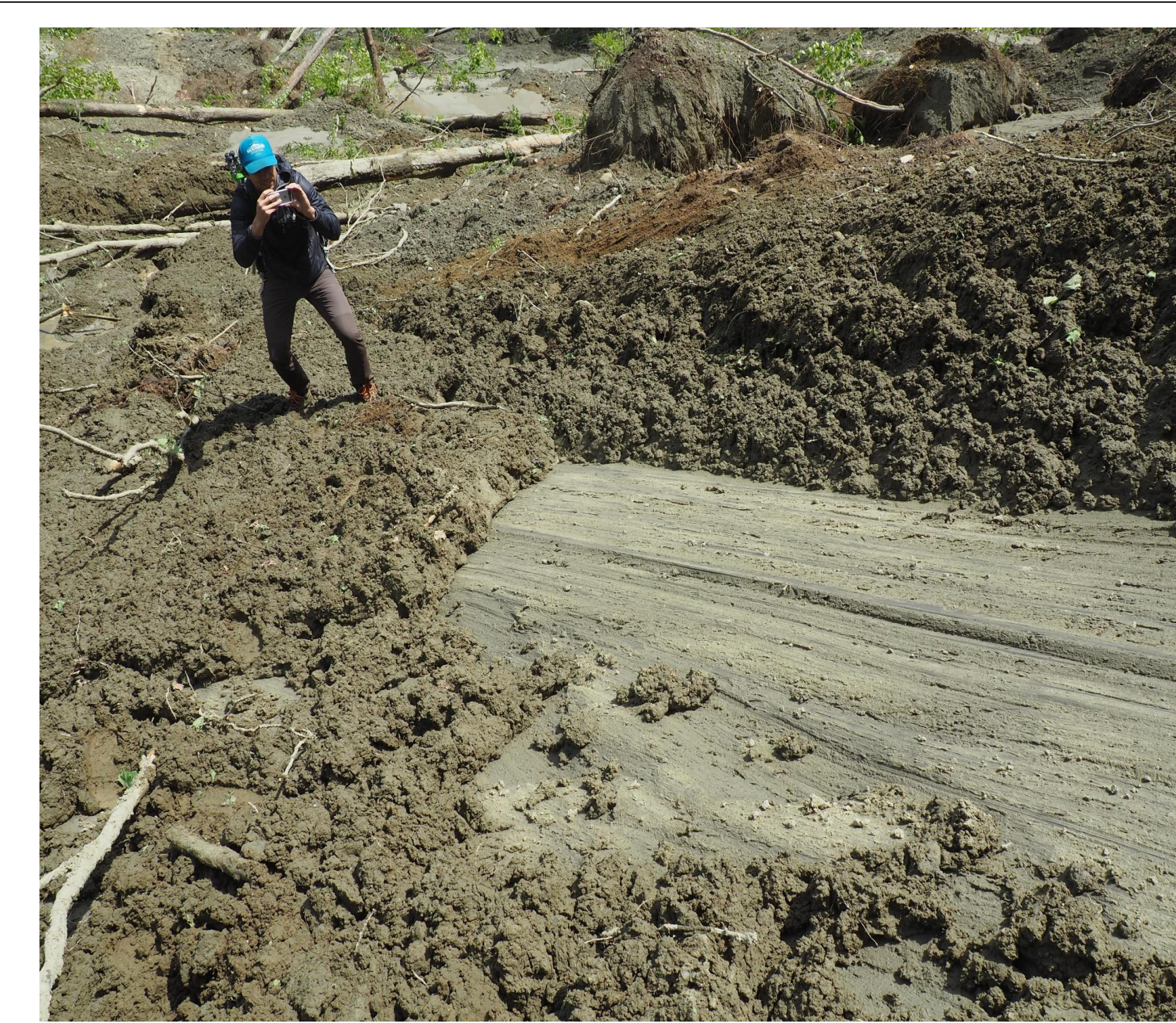
Fig. 5. June 4, 2019: Grooved, striated slip surface beneath sands, silt and debris near the base of the slope. No bedrock was exposed.
