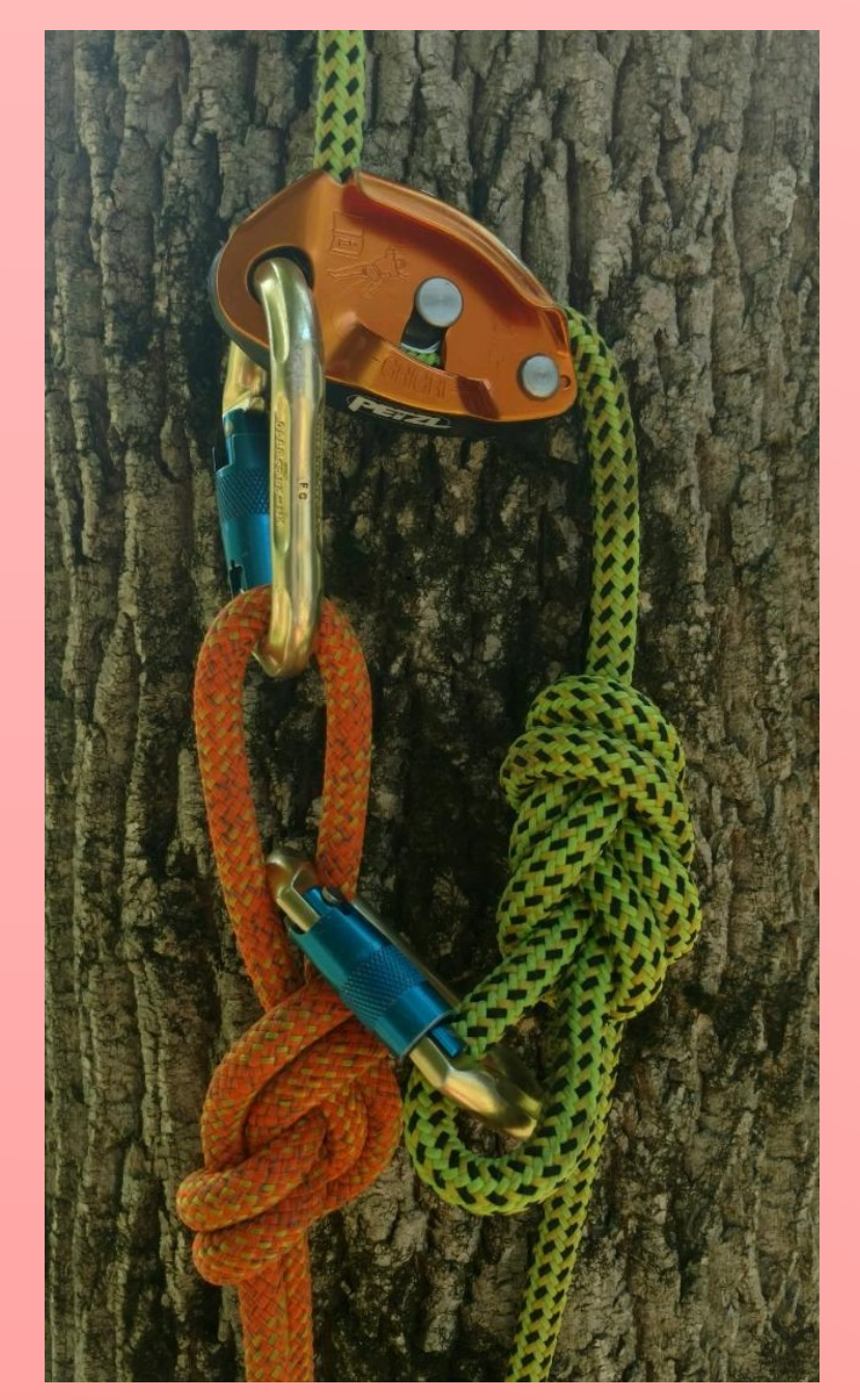
A releasable basal anchor for climber safety (above). Alex Young using sling-shot to get a line over a structural limb (below).
