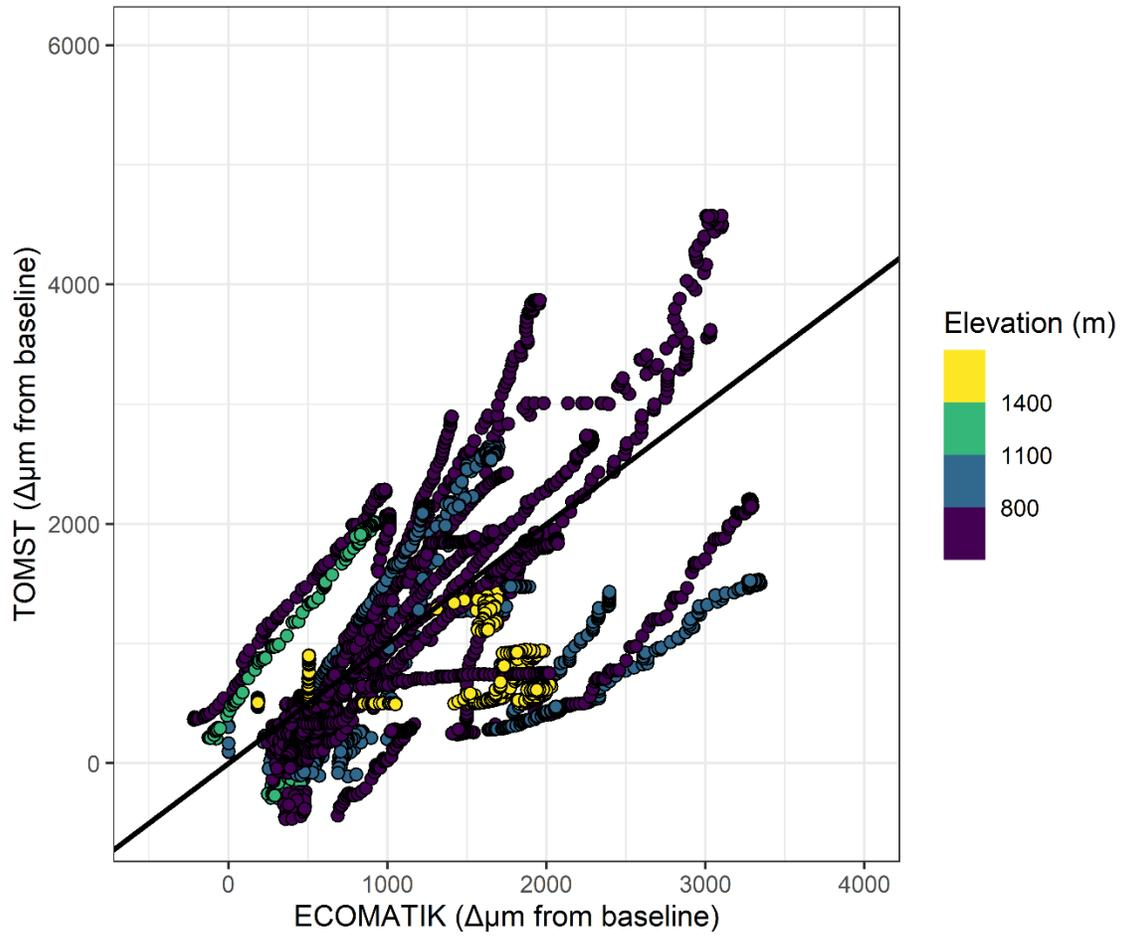
**Figure 6:** Comparison of TOMST and Ecomatik growth measurements partitioned by site elevation. Solid line indicates 1:1 line.
