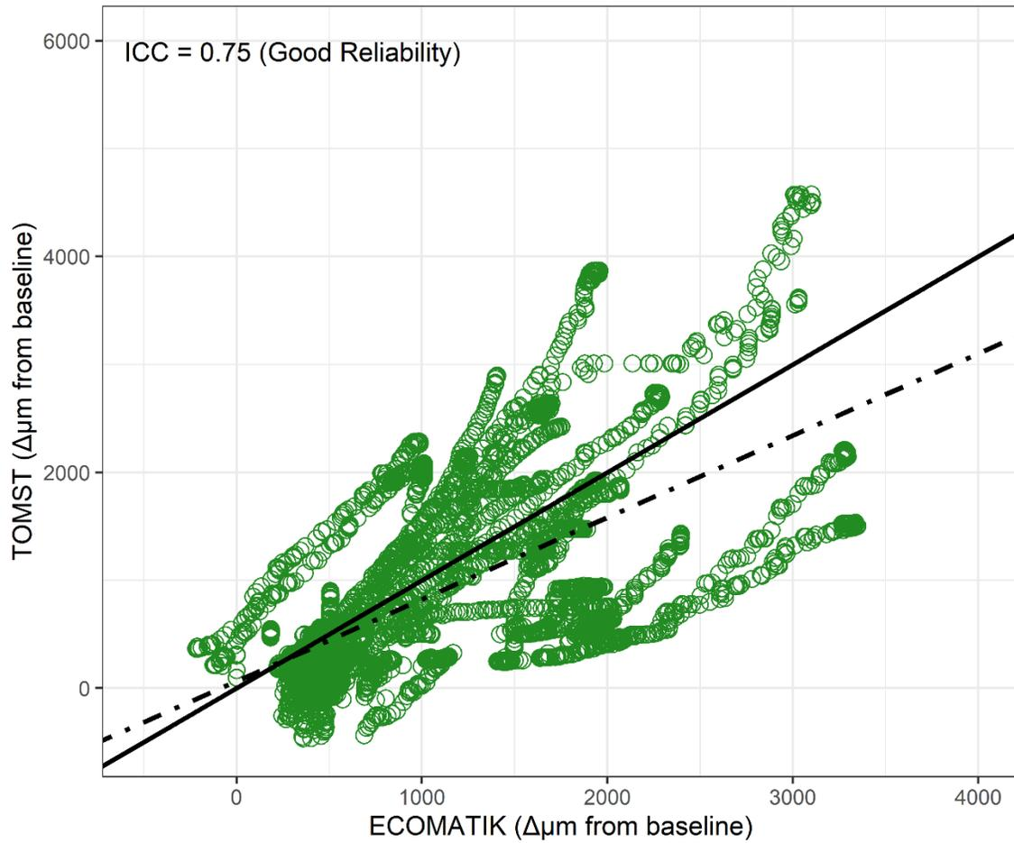
**Figure 5:** Direct sensor measurement comparison between Ecomatik (x-axis) and TOMST (y-axis) dendrometers. Interclass Correlation Coefficient (ICC) of 0.75 indicates good agreement between the two sensors. The solid line indicates the 1:1 line and dotted line indicates best linear fit.
