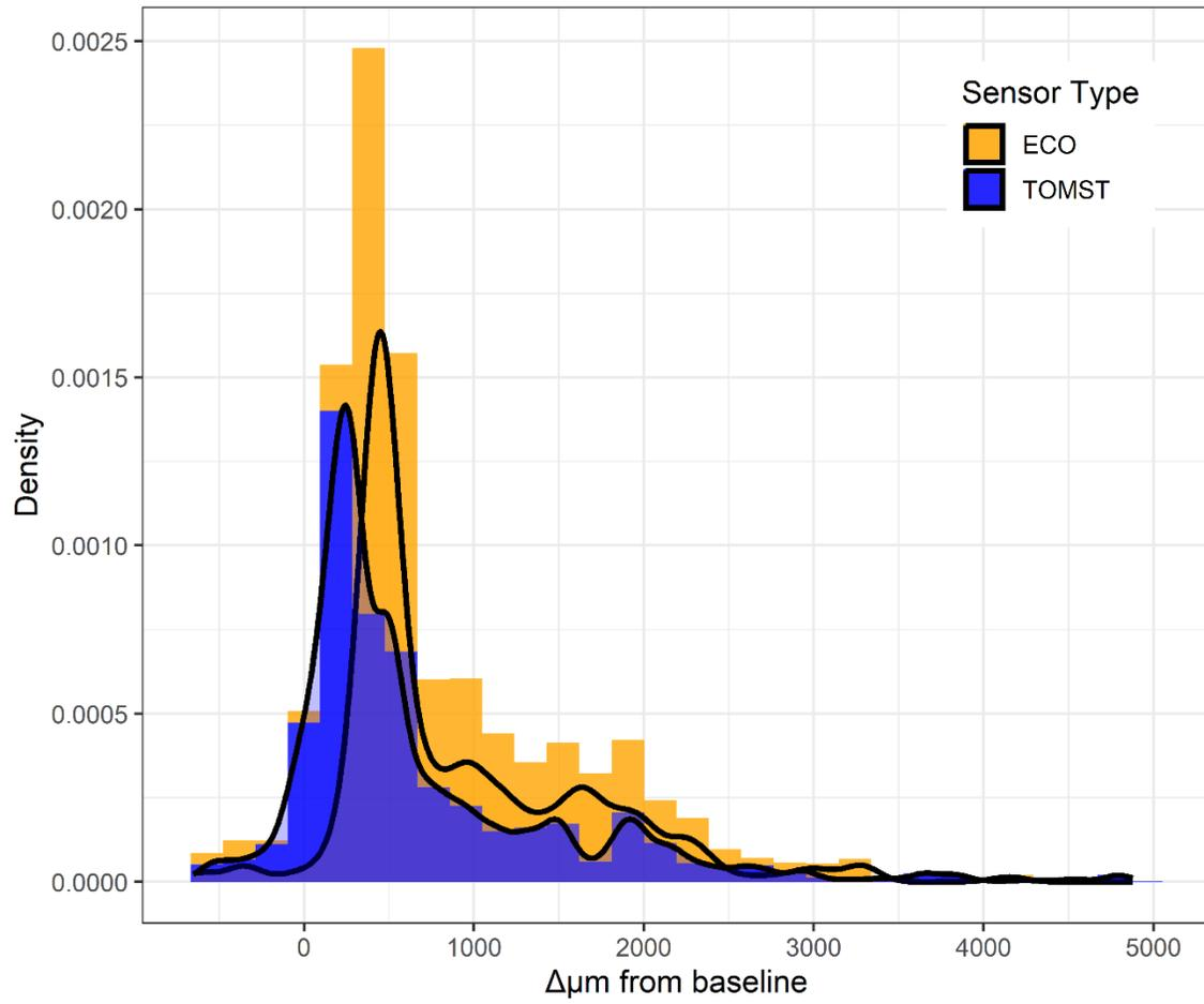
**Figure 3:** Growth measurement histogram for the two dendrometer types. Line indicates measurement density distributions.
