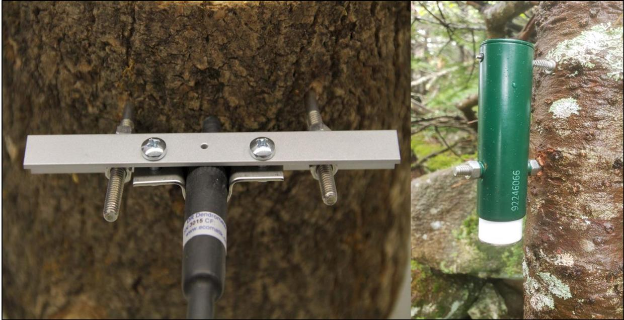
**Figure 2:** Images of the two dendrometer models used in this study. Left: Ecomatik point dendrometer with a cost of approximately \$400. Right: TOMST point dendrometer with built in temperature sensor with an approximate cost of \$100.
