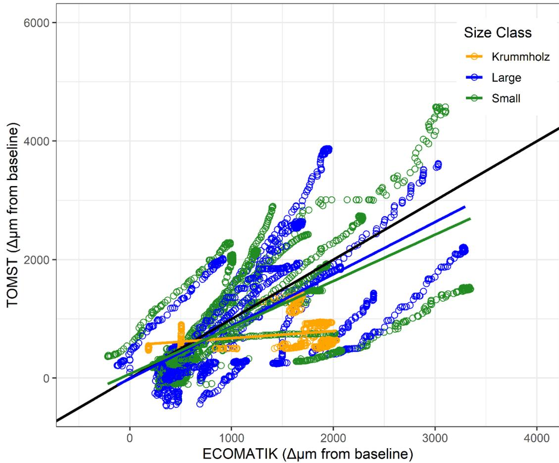
**Figure 7:** Comparison of TOMST and Ecomatik growth measurements partitioned by tree size class. Solid line indicates 1:1 line. Colored solid lines indicate best linear fits by tree size class.
